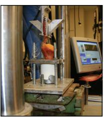
This is the rotator cuff tendon being repaired in a cadaver model. Once it is repaired it is mounted to a servohydraulic machine and tested.
